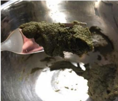
**Fig. 1** 2g KP combined with 10g cold water (20% Solution) producing a thick gel.
