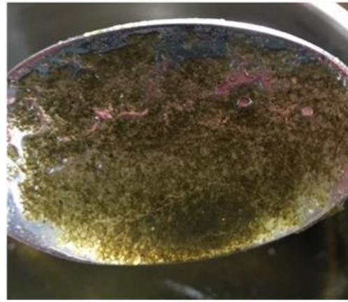
**Fig. 4** Close up of consistency of resulting mixture shown in figure 3 (inhomogeneous solution with visible KP particles and intense green colouration).
