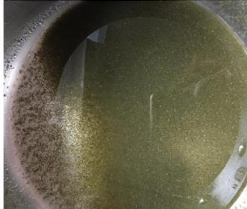
**Fig. 2** 8g KP combined with 100g cold water (8% solution).
