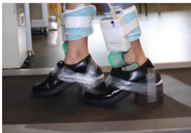
**Figure 1:** Heels made from ethyl vinyl acetate 9 cm (right) and 3 cm (left), respectively.
